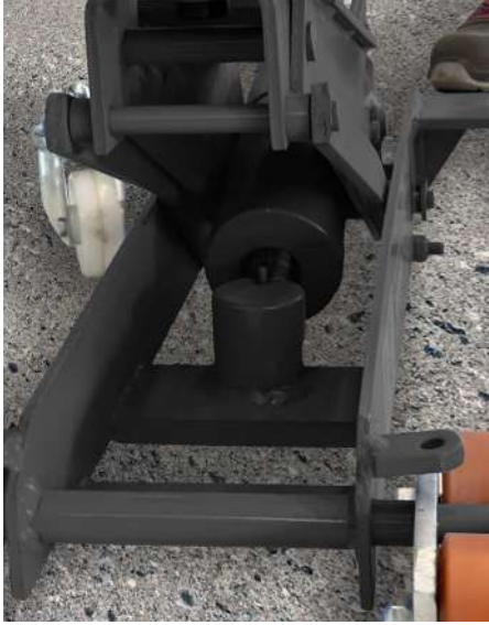
AUTOMATIC END STROKE SAFETY VALVE
