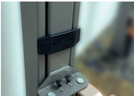
PROTECTION OF THE SPINDLE AND IMPACT PROTECTION FOR CAR DOORS
