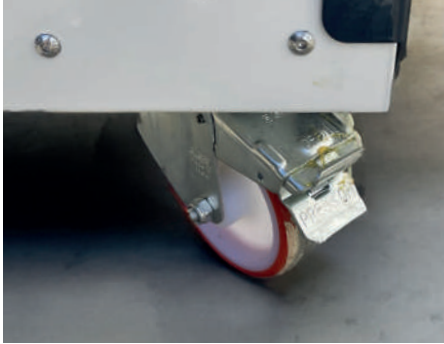
SWIVEL REAR WHEELS WITH BRAKE
