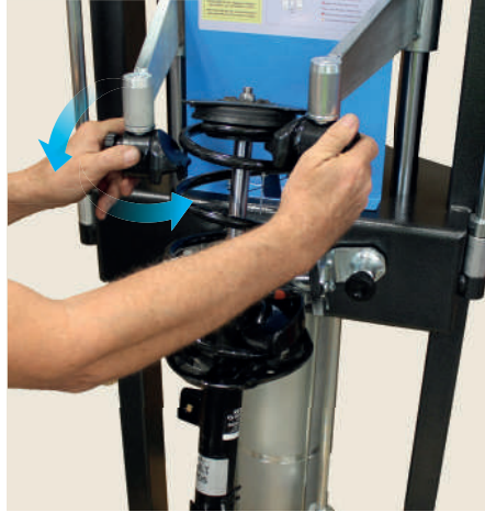
UPPER FLOATING CLAMPS , these floating clamps allow a better grip on the spring, dynamically adapting during the different compression phases.
