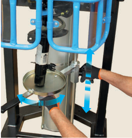
SUPPORT FOR THE HYDRAULIC PART OF THE SHOCK ABSORBER ADJUSTABLE IN HEIGHT AND 180° ADJUSTABLE
