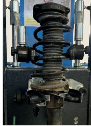
POSSIBILITY OF DOUBLE POSITIONING of the bracket to have more space and stroke for spring compression.
