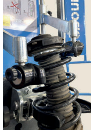
THESE FLOATING CLAMPS allow a better grip on the spring, dynamically adapting during the different compression.
