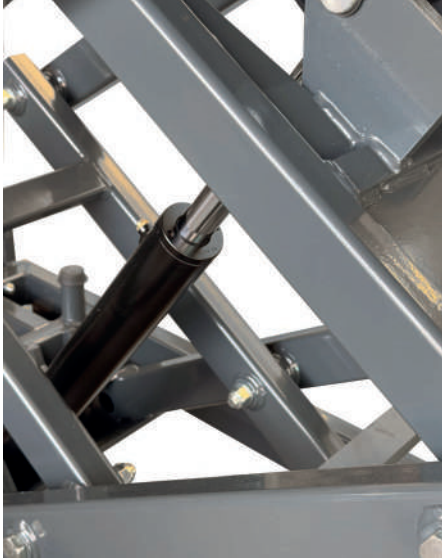
HYDRAULIC CYLINDER WITH GROUND PISTON AND INTEGRATED PARACHUTE VALVE for safety in the event of hydraulic hose rupture
